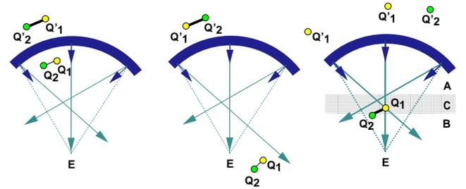
**Figure 8** Behavior of reflections on concave reflectors.
