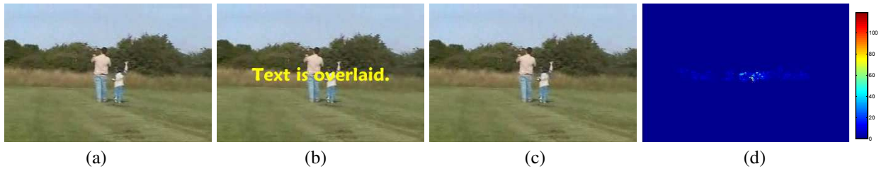
Figure 13: Comparison of the ground truth and the text removal result. (a) a frame from the original video, (b) a text is overlaid on the original video, (c) result of text removal, and (d) absolute intensity difference between the original and result frame.
