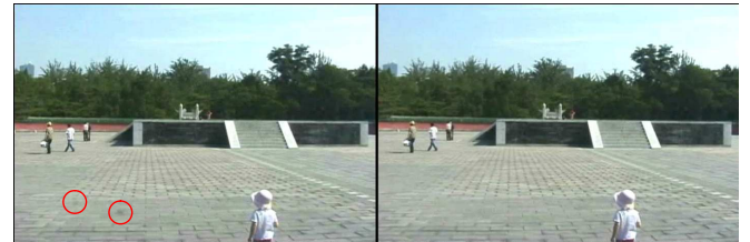
Figure 11: Sensor dust removal. Left: Spots on the camera lens are visible in the original video. Right: The spots are removed from the entire sequence by masking out the spot areas and applying our video completion method.
