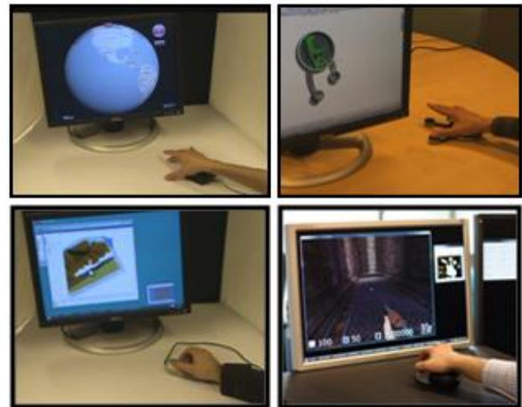
Figure 16. Applications running with our MT mice. Clockwise from top-left: manipulating Virtual Earth, precise modeling in SolidWorks, controlling a FPS game and browsing using a desktop mockup.
