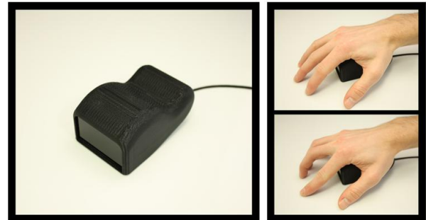
Figure 10. Side Mouse is augmented with a proximity-sensing technique called SideSight, which enables multi-finger sensing on the surface around the device.
